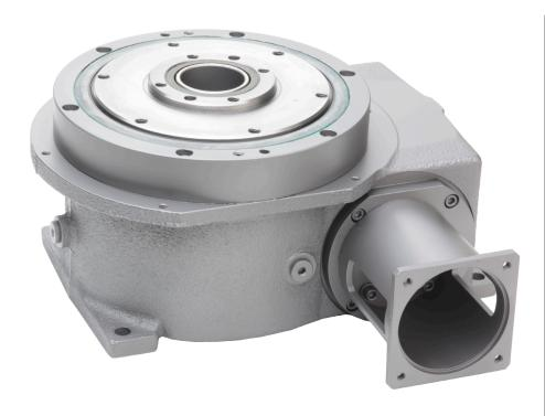
The Cyclo-Index 3400DTW is a servo-driven rotary dial table designed for applications that require flexible motion, high accuracy, and low maintenance. The dial is supported by precision crosscontact radial bearings, and the driving mechanism can offer as little as zero backlash. This robust gearbox features a large, center through-hole to feed electrical, fluid power, or other lines.
